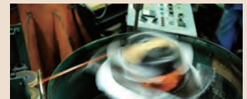
Winding of copper wire to the rotor by automatic winding machine
