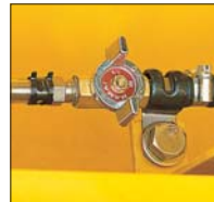
Fuel Drain Valve
