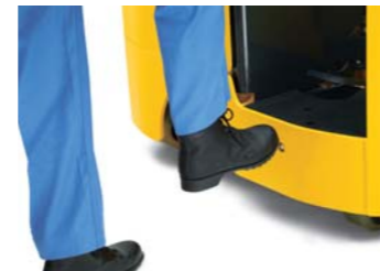
Travel and lifting are stopped when the operators leaves the compartment
