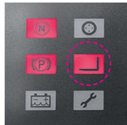
The lifting work interlock is displayed on the monitoring system
