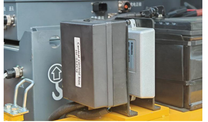
With VCU and independent control box
