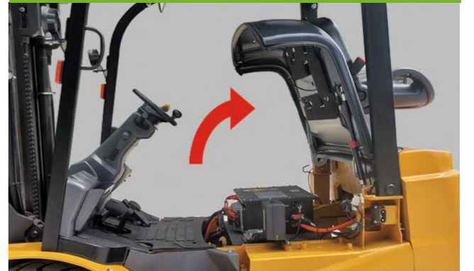
Open the hood at a large angle for easy maintenance
