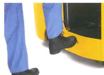
Travel and lifting are stopped when the operators leaves the compartment
