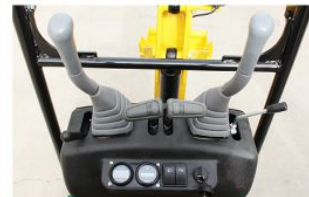
Operating rod Hydraulic pilot operation
