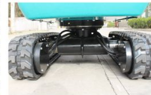
Retractable track Convenient for narrow space operation
