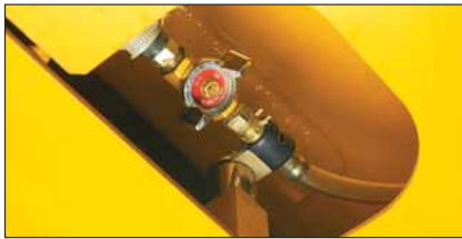
Fuel drain valve
