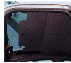
Sun visor protects the operator from overhead sunlight
