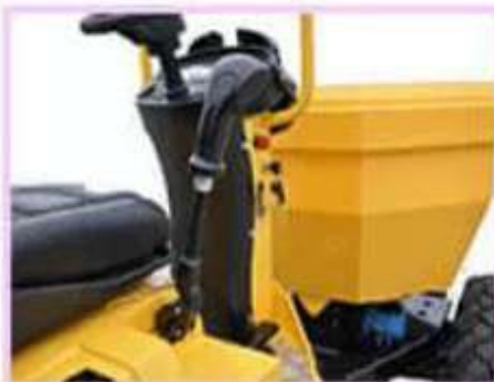
Walking reversing mechanism with a neutral locking function ensures safe start of the machine
