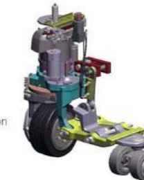
Automatic suspension incorporating new control linkage
