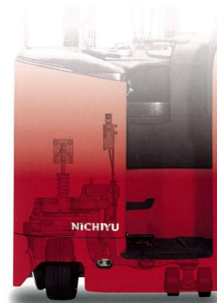
Automatic suspension incorporating new control linkage
